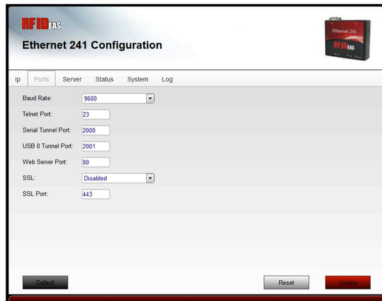
The screenshot displays the 'Ethernet 241 Configuration' web interface. At the top, there is a navigation menu with tabs for 'Ip', 'Ports', 'Server', 'Status', 'System', and 'Log'. The 'Ports' tab is currently selected. The configuration fields are as follows:
