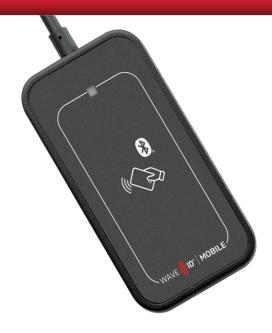
The WAVE ID Mobile Mini combines a multi-frequency programmable card reader with integrated **Bluetooth®** low energy technology. In addition to reading both proximity (125 kHz) and contactless smart cards (13.56 MHz), it also works with BLE-enabled devices to read mobile credentials in end-user applications such as in-building location and secure authentication.
