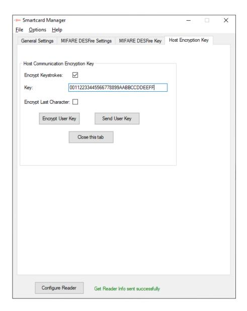
Keystroke encryption button will enable/disable encryption of keystrokes. The key is currently a 16-byte (32 hexadecimal characters) field, for AES-128 encryption (initial div input of 0x00). Other key types may be available in the future.
