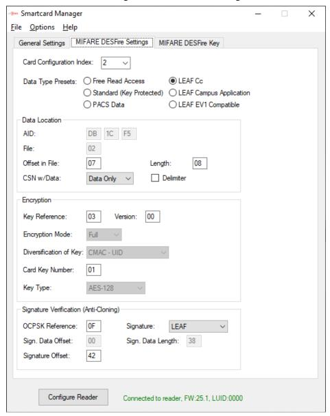
The Data Type Presets at the top are quick presets for common uses. For example, the LEAF Cc and LEAF EV1 Compatible presets will fill in the fields to read the Badge ID from a standard LEAF card. The other options are for more customizable data selection.
