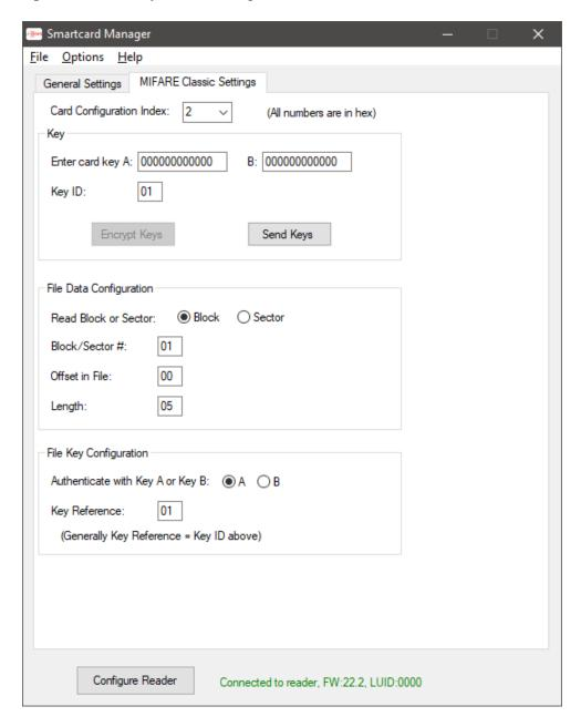
Note: The reader firmware has been extended to be able to keystroke up to 48 bytes of data (a typical sector of MIFARE Classic). The SDK (API) interface, however, still has a maximum of 32 bytes. This is only noticeable if the configured length is more than 32 (hexadecimal 20), and the pcProxConfig utility (or similar application using our DLL) is used to retrieve data. The first 32 bytes are returned, and it reports a maximum of 255 bits of data.
