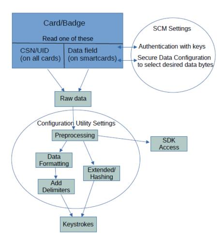
The Smartcard Manager will inform the reader what data bytes to read and what keys are needed to access that data. Then pcProxConfig or the rf IDEAS Configuration Utility can be used for formatting of that data, to get the desired output for keystrokes or accessing by SDK. Data in SDK undergoes less processing than keystroke data.
