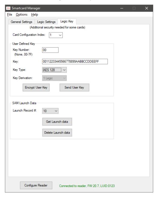
The key is entered on this tab, and stored at location Key Number in the LEGIC chip. The key cannot be read back. If desired, the key can be encrypted after it is entered. Thereafter it will be displayed in the encrypted form, stored in the configuration file as encrypted (if a configuration file is created), and it is sent encrypted over USB to the reader.
