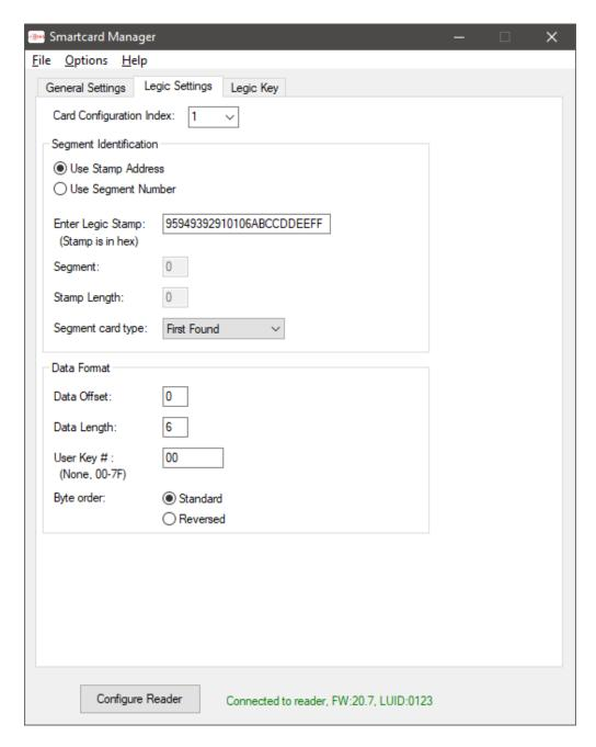
A LEGIC segment can be addressed by the Stamp Address, or by the segment number. When using the segment number, an optional Stamp Length field is available. Entering this will keep the data consistent if both LEGIC advant and prime cards are being used, as the prime card includes the stamp with the card data, while the advant does not.
