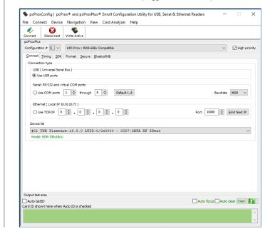
The Model number **RDR-305x1BxU** must be displayed in green font as shown, indicating that the reader is connected. If it is not, then click the "Connect" icon below the top navigation bar. Next, select the Configuration #3 with the dropdown box and then select Safetrust from the dropdown box to the right. Note: If Safetrust doesn't show up, you may be using the wrong version of pcProxConfig, or you may have the wrong reader.
